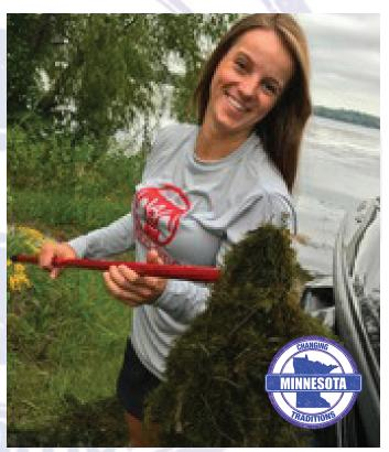
The simple, yet ingenious, device is a combination hook and scraper/cutter on a 4-foot handle that allows the user to gather and pull clumps of vegetation from their rig without marring the finish of the boat or trailer.
