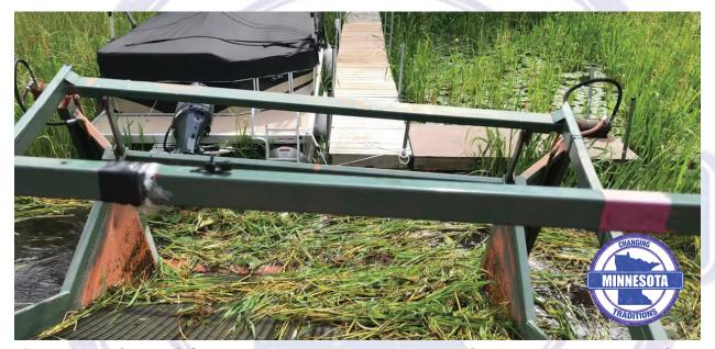
Cutting a channel for private property access under a DNR permit to do so. The sickle bar cuts the plants and the front conveyor brings them onboard and drops them onto a lower, rear conveyor.
