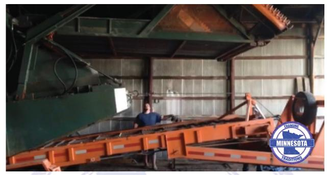
Offloading. The rear conveyor offloads to the trailer which has a live bottom. A typical load is about 5,000 lbs wet weight. The trailer also hauls the harvester to and from the lake.
